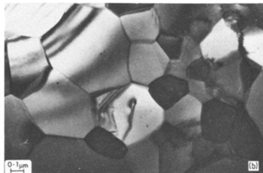
Figure 5 Micrographs (longitudinal sections), showing variation in equiaxed grain size with heat-treatment: (a) reacted 160 h at 750°C; (b) reacted 333 h at 780°C and 144 h at 900°C.
